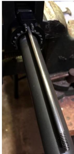
Once the BCG is installed, cycle it a few times to ensure it moves freely. The BCG should be lubricated as normal for ease of movement inside the upper receiver and you may include a light film to the push rod in case there is any incidental contact. If all is well, remount the upper receiver assembly in the Action Block and load both back into the bench vise. The push rod should be aligned parallel with the barrel center and look something like what is shown in the photo above right.
