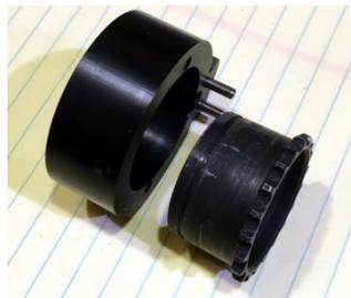
When this sub-assembly is in place on the barrel, re-torque the barrel nut as described earlier such that the marked lug recess is properly aligned with the gas tube hole.
